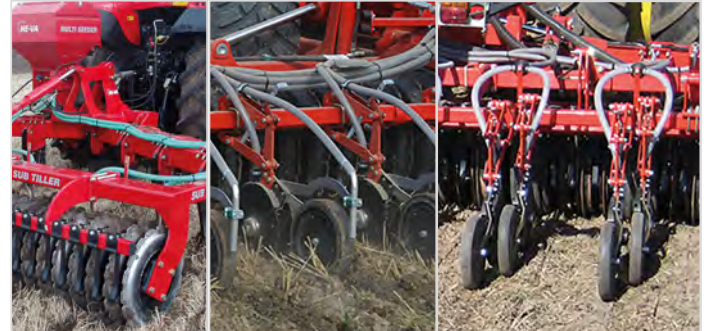
Seeding with disc coulters (12 cm btw./coulters) with 75 mm wide depth/press wheel. Placed in 2 rows around centre line of the tine, after packer roller.
