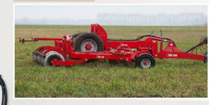
Trailed Sub-Tillers are rated to work with higher horsepower tractors up to 600 hp.
