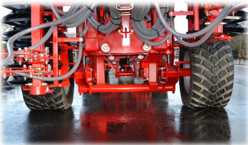
Photo no. 2. Transport legs are resting on the wheel frame.
