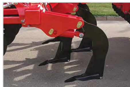
Tine design in Combi-Tiller MKII and Combi-Disc.
