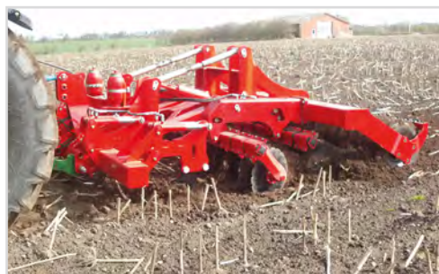
Combi-Disc with the tines in max. working depth, ensuring a soil loosening, cultivation and a consolidation.
