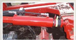
On all models the working depth is adjusted hydraulically from the cabin with the possibility of fixed stop via the distance clips.
