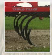
Automatic tine with single spring/auto reset, preloaded for 560 kg, ensures an effective 0 - 30 cm cultivation of even the heaviest soil types.
