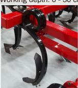
Shear bolt, preloaded for 2,550 kg.
