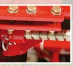
For top soil and for smaller fields, the Ouick-Push stone protecion system is the obvious choice. Once the tine meets a stone, the shearbolt with 8 steps will be cut. The simple procedure of removing the R-clip and pushing the bolt into place again can be done completely without the use of tools and you will quickly be on your way again.
