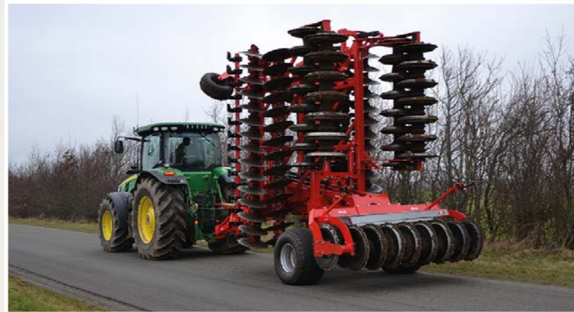
Disc-Roller XL Contour with 2-section disc section and 3-section roller section in transport position (6.50 + 7.50 m)
