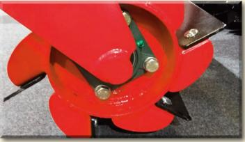
The unique design with a closed tube construction prevents soil and residues from gathering and sticking to the Top-Cutter and ensures a continuous, high degree of efficiency. The six double-sided knives ensure an even and stable workflow. The
