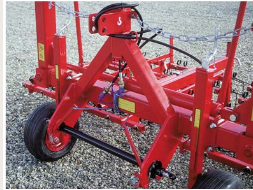
Linkage system of 6.00, 7.50 and 9.00 m. Detachable bar.
