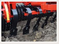
The Spring-Board blades can work individually, but the levelling effect is increased when adding the locking system. This will convert the individual springs into a complete "board".
