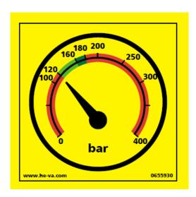
Correct hydraulic pressure on the release system.
