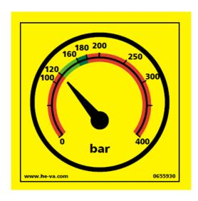
Correct hydraulic pressure on the release system
