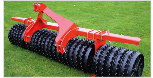
Front-Roller with fixed three-point hitch - not self-steering.
