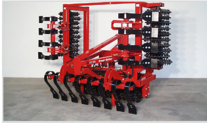
4.00 m Front-Roller with Crosskill, hydraulic folding and Spring-Board.
