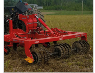
2.50 m with hydr. release system and synchrone Star Roller.
