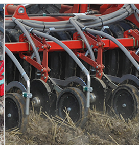
Seeding with disc coulters with 75 mm wide depth/press wheel. 1 row placed in centre line of the tine, after packer roller.
