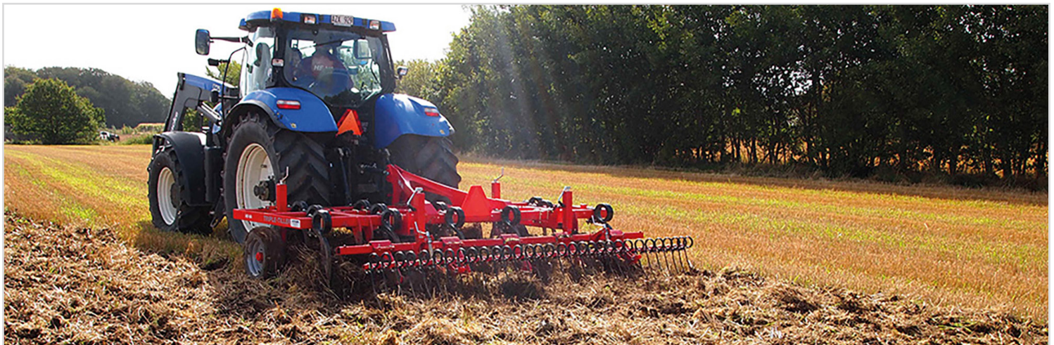
4.00 m Triple-Tiller Airy with spring tines.
