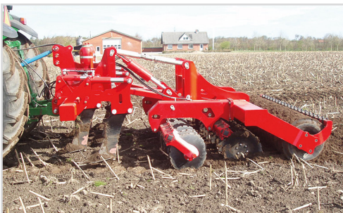
Combi-Disc with the tines lifted free from the soil, meaning that only the Disc-Roller's function is in work.
