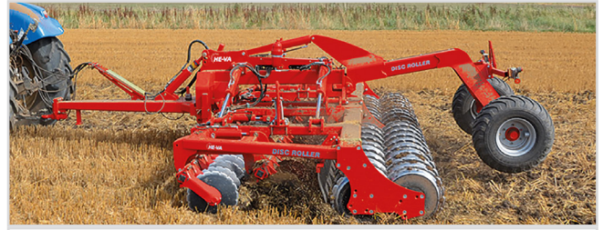
8.00 m Disc-Roller Contour with V-Profile Roller and support wheels.
