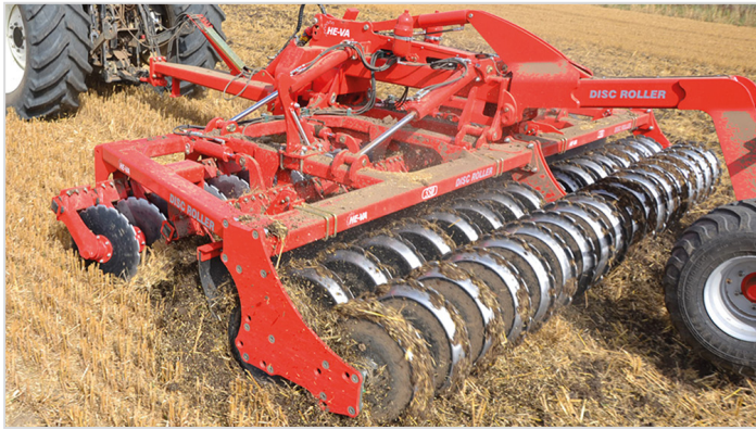
5.50 m Disc-Roller Contour with Twin V-Profile Roller and material damper guard.
