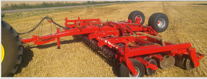
5.50 m Disc-Roller Contour with Twin V-Profile Roller and material damper guard.
