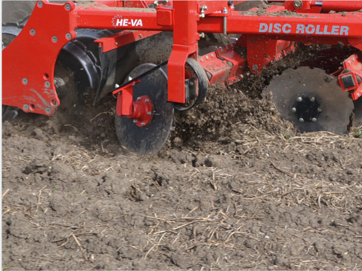
Standard equipment on all models: Adjustable edge disc for retain soil on right side.
