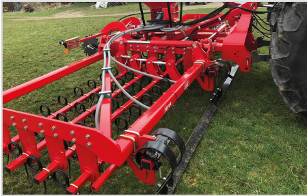
Levelling bar with spindle height adjustment.
