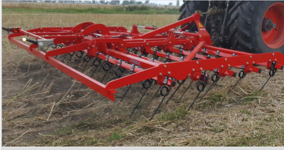
6.00 m Top-Strigle with 5 rows and 16 mm tines.
